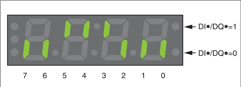
Figure 7.10 Integrated HMI, displaying the signal state of the digital inputs (DI•) and outputs (DQ•)
